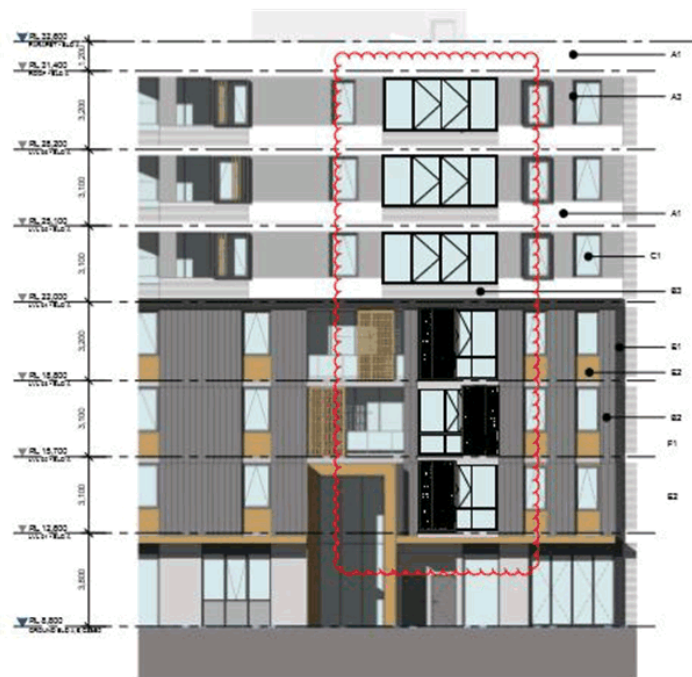
Figure 2. Example of detail of wintergardens on western elevation
